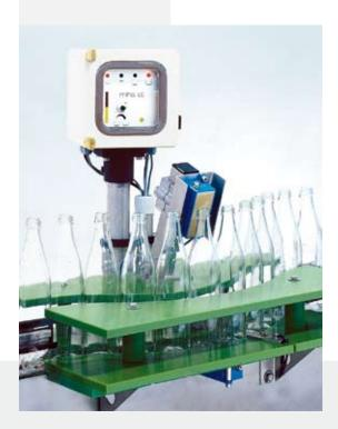
The miho LC Residual Liquid Inspection Unit is a standard feature of bottling plants today.
